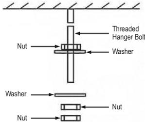
**NOTE:** The hanger bolts, nuts, and washers are field supplied. Install the washer with cushion so that the insulation faces downward.
