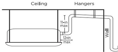
Use an auxiliary condensate pump with float valve for vertical height greater than of 11-in. (280 mm) above the unit drainage port. A float valve is recommended to shut off the system if the auxiliary pump fails.
