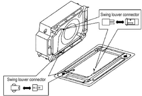
6. Find the four (4) height adjustment screws located on the corners of the decorative grille. Use the four (4) height adjustment screws to adjust gap between decorative grille and Ceiling Cassette body so that gap is reduced to 1/4-in (6mm) to 3/8-in (9mm). Make certain the decorative grille is not distorted by excessive tightening.
