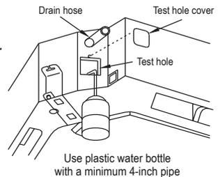
**Note:** This unit is equipped with a safety float switch to de-energize the compressor if the water level gets too high.
