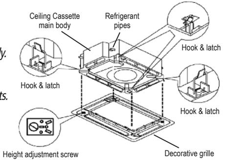
**Note:** Be careful not to pinch the swing louver motor wires between the decorative grille and ceiling cassette main body.
